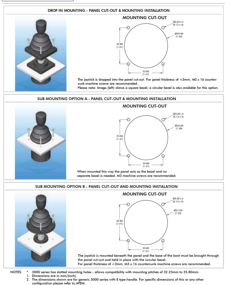
3. When sub panel mounting, great care should be taken not to damage the boot, or any of the mechanism under the boot. All panel cut-outs should be free from sharp edges and debris that may damage the boot.
